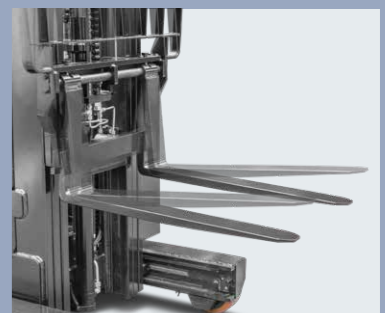
Forks can tilt forward/backward for easy loading
